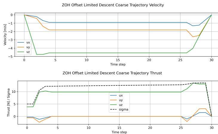
Fig. 1 Generated trajectory velocity and thrust for the offset limited descent.
